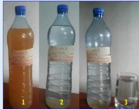
SaferEx - Multi-action Water Purifier used in treatment and recovery of safe water from muddy, heavy metal and pathogen infested raw borehole water from Okposi Town, Ohaozara L.G.A, Ebonyi State, Nigeria (In situ treatment).
