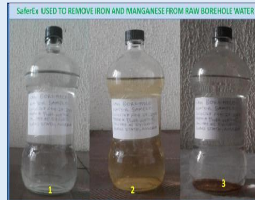
Raw borehole water at Oyigbo town, Rivers State, Nigeria analyzed to contain high Iron and Manganese but remains clear in appearance (Collected from a water packaging factory).
