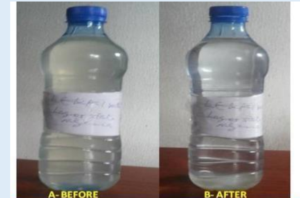
SaferEx in situ treatment of household borehole water from LEKKI, Lagos State, Nigeria analyzed and contains pathogens, metals and salts. A -Before treatment with SaferEx B -After treatment with SaferEx with sediments; rid of pathogens, salts and unwanted metals prior to filtration (after < 45 minutes).
